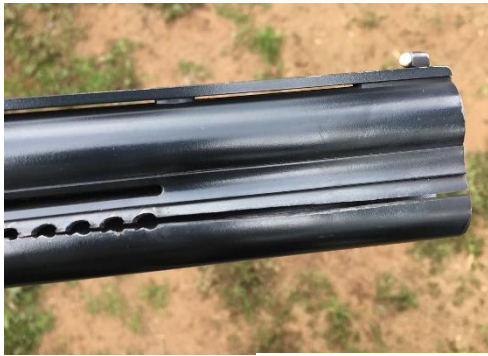
Split Barrel due to obstruction
