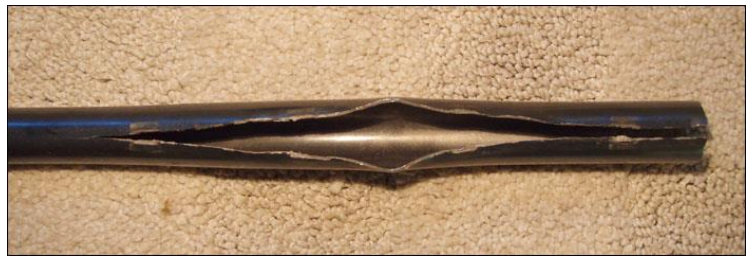
Split Barrel due to obstruction
