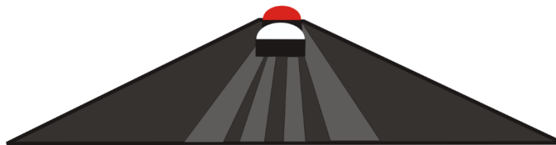
Straight and correct figure 8 alignment along the barrel
